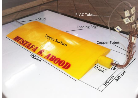
Fig 2: Single Element Airfoil Test Model Used in Wind Tunnel
