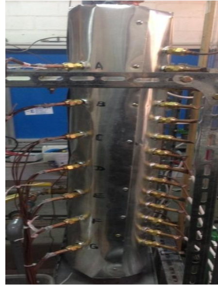
Fig (2): Sub-millimeters bubbles injection system and temperature measurement taps
