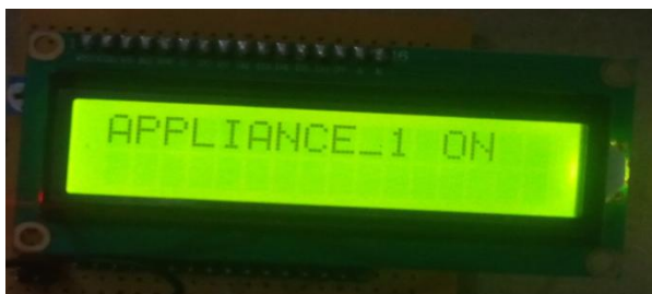
Fig 7 LCD indicating the ON status of Appliance 1
