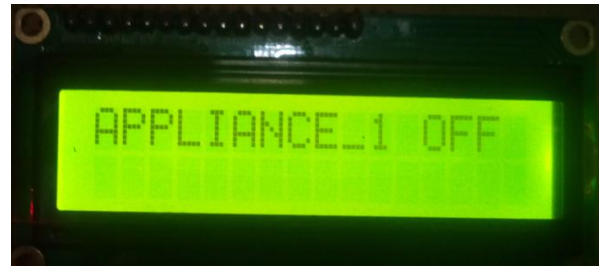
Fig 8 LCD indicating the OFF status of Appliance 1
