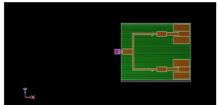
Fig. 6: 3-D structure of 1:2 Patch Antenna Array with DGS
