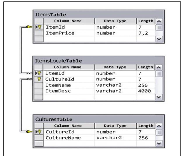
Figure 19: Items Database Table Structure - Good Design
