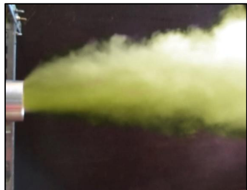
(b) Positive pitch vectoring R/d = 1.174647 , h/d = 0.02941 , m_s/m_p = 0.06568
