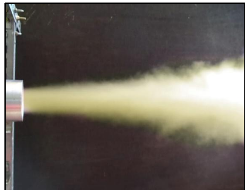
(a) Non-vectored primary flow, R/d = 1.174647 , h/d = 0.02941 , m_s/m_p = 0
