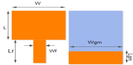
Figure 3. Partial ground plane patch antenna ( W=8 mm, L=5 mm, W_f=1.6 mm, f=10 mm, W_{gm}=17.6 mm and L_{gm}=6 mm) [12].
