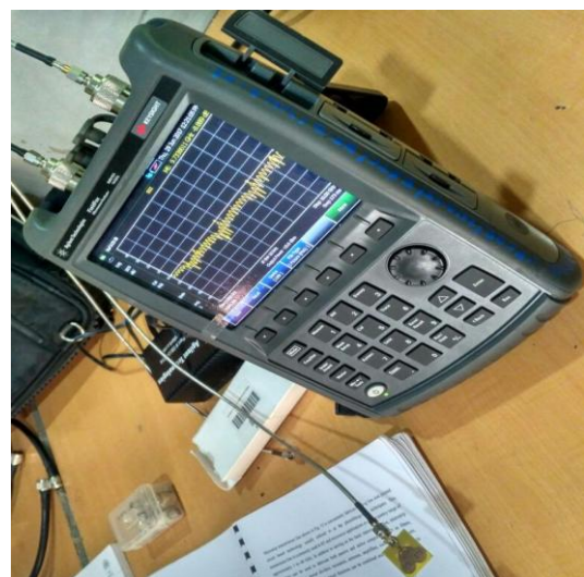
Figure 6(b): S 11 Measurement Setup
