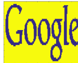
Fig. 4: Extracted watermark image (50×25) from watermarked video frame with NCC = 1
