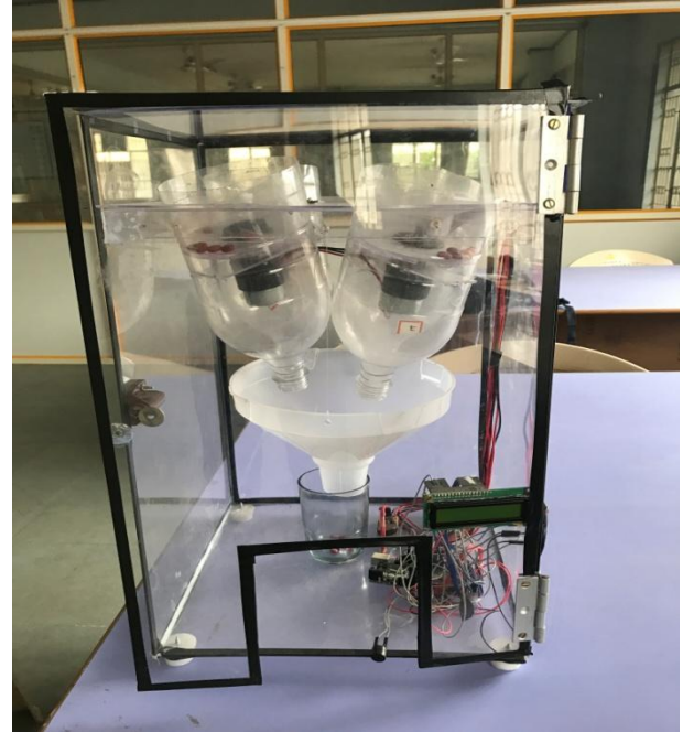
Fig. 4 Front view of medical dispenser and reminder
