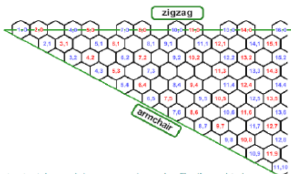
Fig12: Single Walled Carbon Nanotubes (Graphene) Sheet with the possible rolling designs (Zigzag and Armchair)
