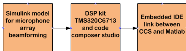
Fig.3: The requirements for implementation the real time signal processing system when using DSP kit
