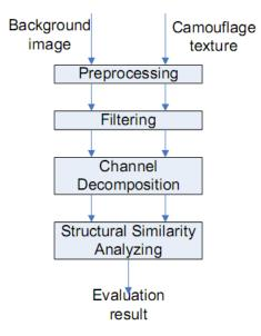
Fist, a variety of basic operations is performed to eliminate distortions from background image and camouflage texture. And a low-pass filter simulating the point spread function of the eye optics may be applied. Second, the luminance of camouflage texture and background image is compared as follows:
