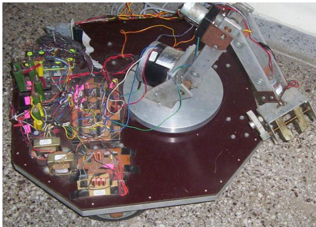
Fig. 2 : Robot with the gripper as the end-effector
