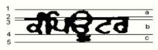
Figure 4: a) Upper zone from line number 1 to 2, b) Middle Zone from line number 3 to 4, c) lower zone from line number 4 to 5.
