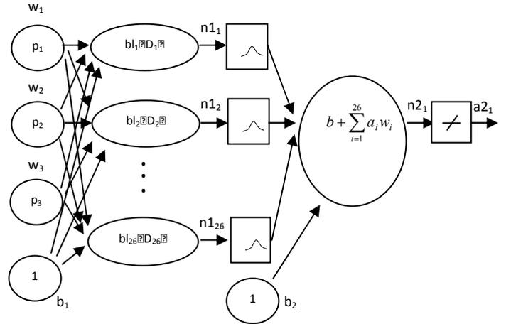
Fig. 1. RBF architecture used to model of lead acid battery (number of input variable 3, amount of data 26, single target)
