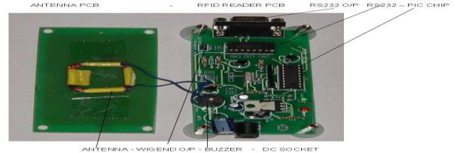
Figure 3 Inside RFID Reader
