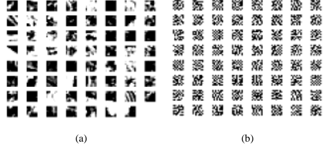
Figure 5. (a) Basis functions, and (b) orthogonalized basis functions.
