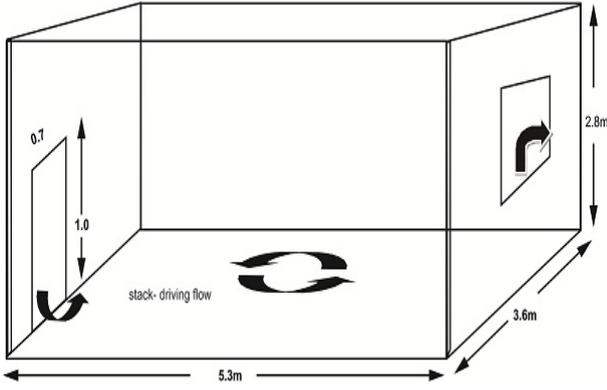
**Fig 3: Schematic diagram of airflow process inside unstratified cross ventilated rectangular building with two openings.**
