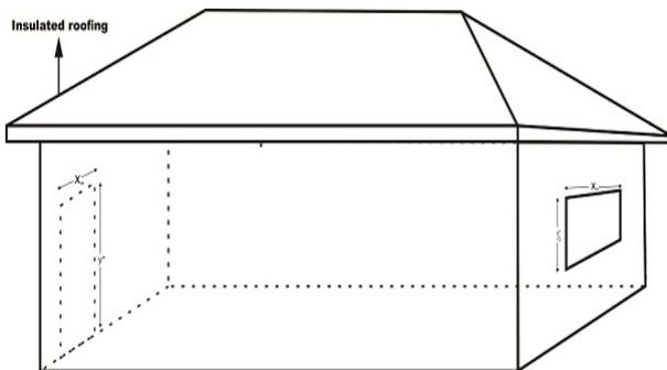
Figure 1: Diagram of un-stratified cross ventilated rectangular building with two openings.
