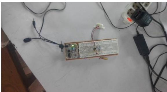
Figure 5. Testing Mobile Detector without a Jammer on Bread Board.
