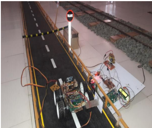
Fig 5.1 Developed model of the toll gate in closed state
