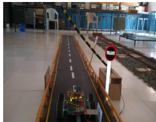
Fig 5.4 Toll gate open after the RF validity is verified
