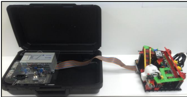
Figure 10: Wired Connection between PLC and System
