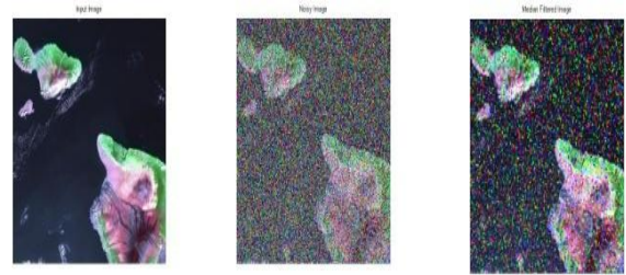
a) Input Image4 b) Noisy Image c) Median Filter
