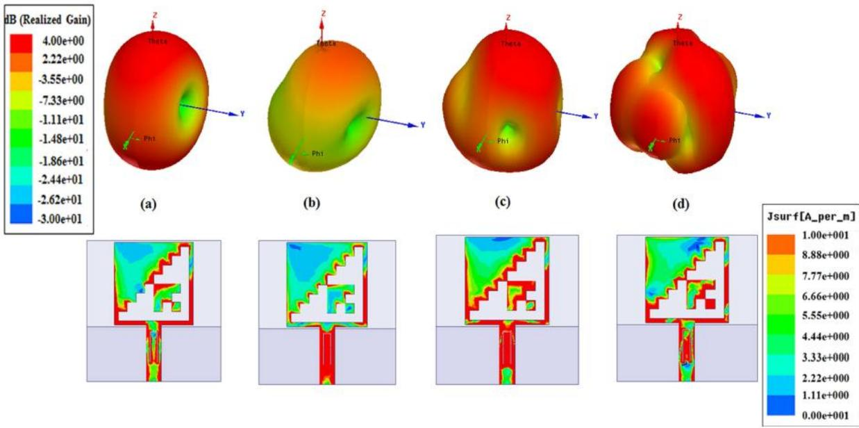
Figure 1.8: Simulated 3D radiation patterns for MSSF antenna at (a) 4 GHz (b) 5.5 GHz (c) 6.2 GHz (d) 8.7 GHz.
