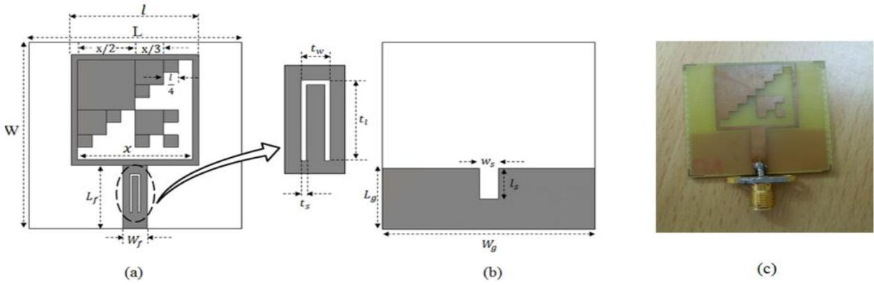
Figure 1.2: Geometry of MSSF antenna (a) Front view (b) Rear view (c) Photograph.
