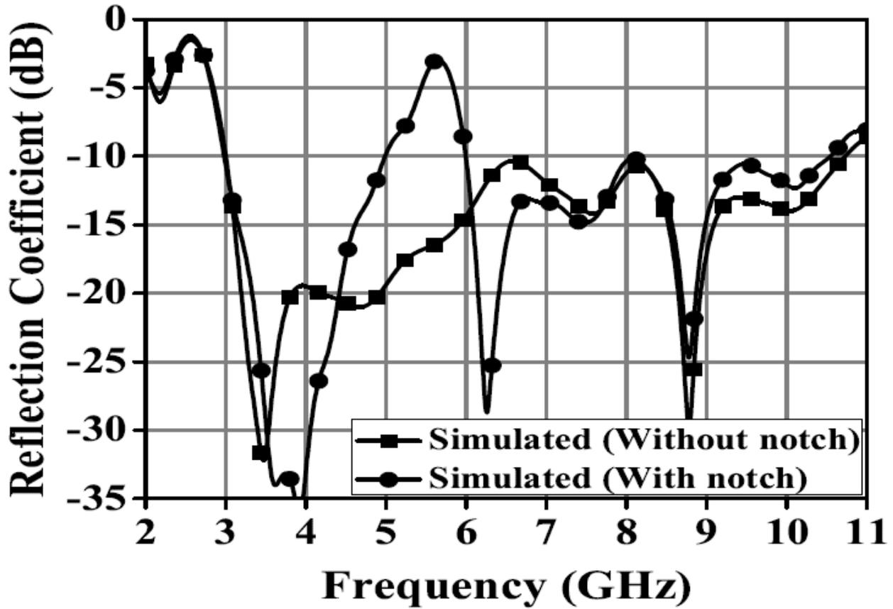
Figure 1.7: Simulated reflection coefficients of MSSF antenna for with and without notch.
