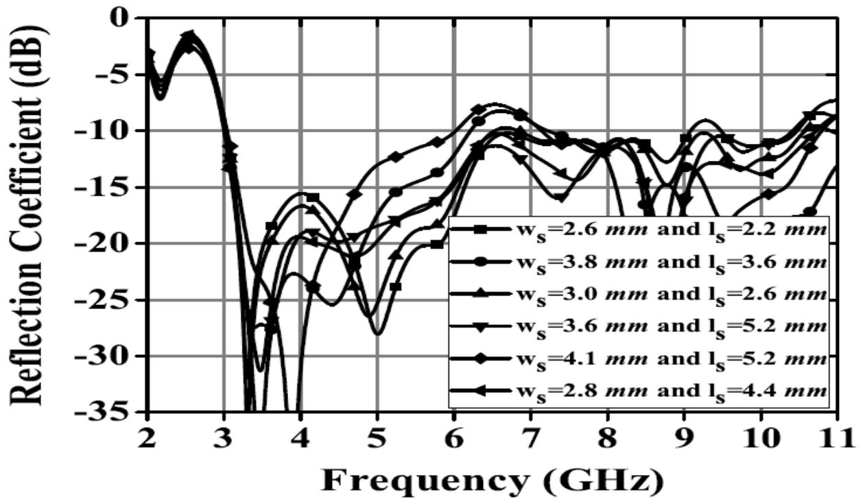
Figure 1.5: Simulated reflection coefficients of MSSF antenna for different configuration of grooved ground plane.
