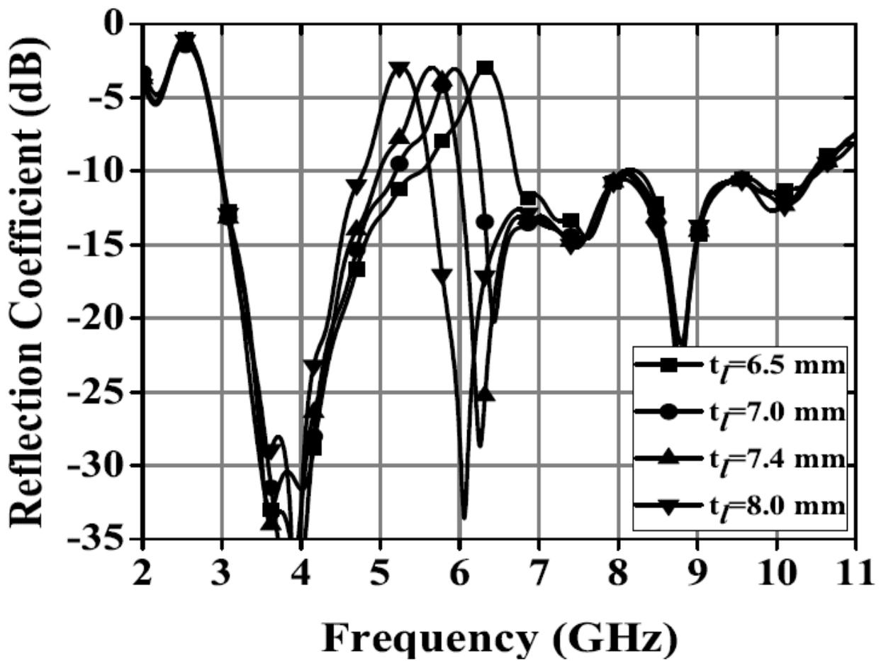
Figure 1.6: Simulated reflection coefficients of MSSF antenna for length  $t_l$  of band notch slot.
