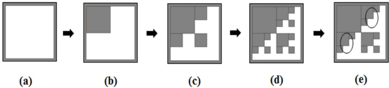
Figure 1.3: MSSF geometry and its different stages (a) Basic geometry (b) First iteration (c) Second iteration (d) Third iteration (e) Modified geometry
