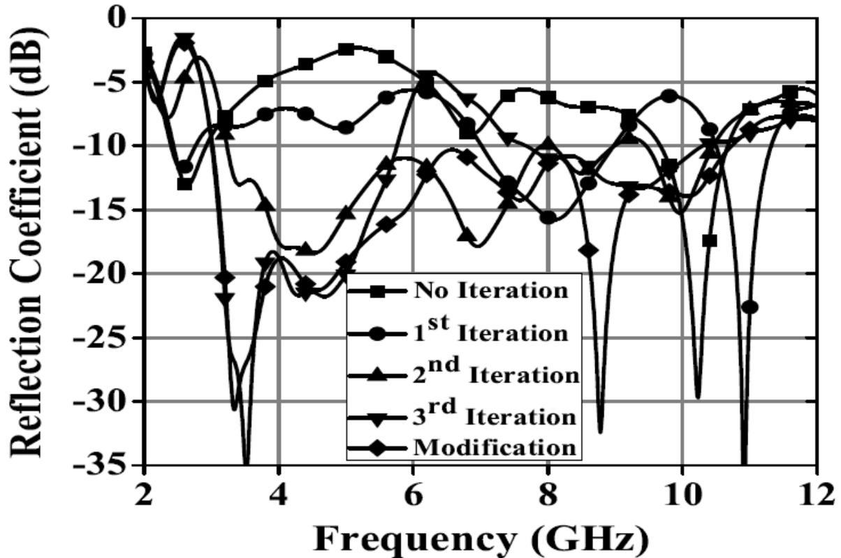
Figure 1.4: Simulated reflection coefficients of MSSF antenna for different iteration.
