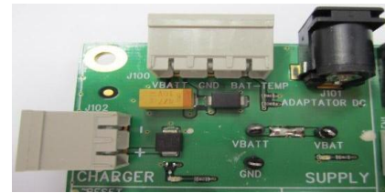
Figure 8: Sierra Wireless GSM Power supply unit
