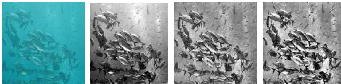
d) Original See image e) CLAHE enhanced image f) contrast adjustment g) Dual Enhancement
