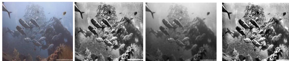
h) Original Bubble_vision image i) CLAHE enhanced image j) contrast adjustment k) Dual Enhancement
