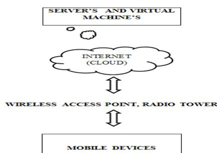
Figure 1: Mobile Computing Architecture
