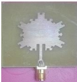
Figure 8: Fabricated structure of proposed antenna
