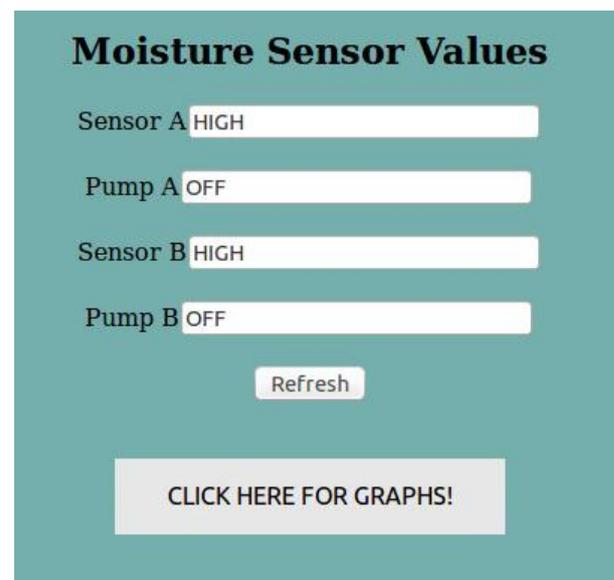
Figure 3: Webpage showing sprinkler and soil moisture status
