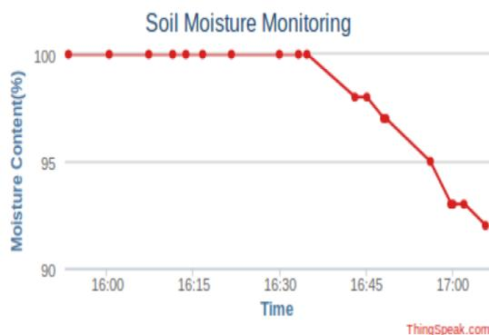
Figure 6. Graph of Sensor B: Inserted in over irrigated soil
