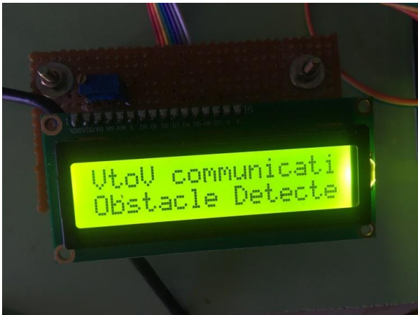
Fig7. LCD Showing Warning Message
