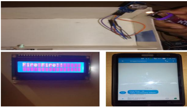
Figure 12: Live demo-gas/fire detection
