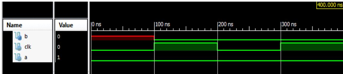
Fig. 4.3 Test bench waveforms of Latch
