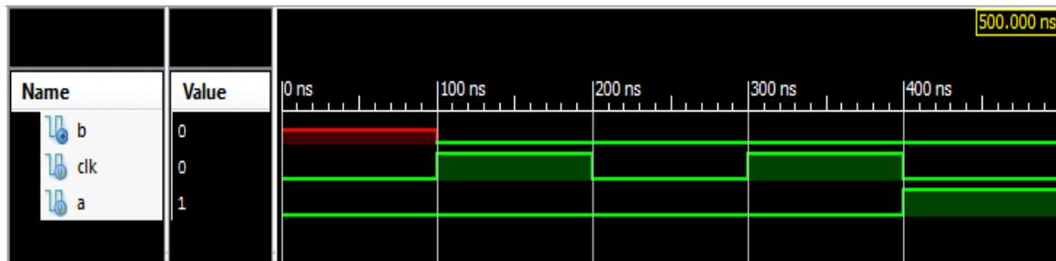
Fig. 4.4 Test bench waveforms of Shadow Latch
