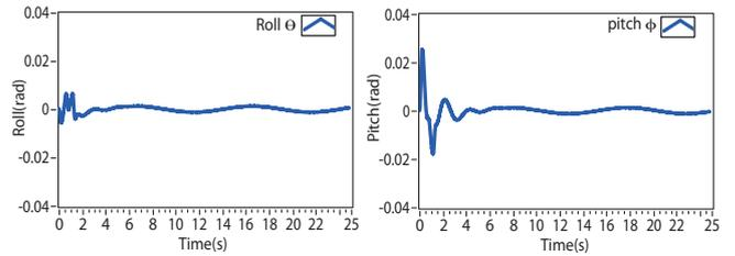
Fig. 13. The attitude signals generated to track the ellipse trajectory. (a) the roll response. (b) the pitch response.
