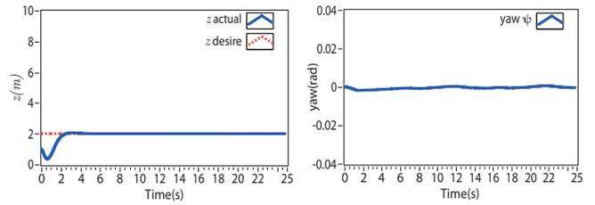
Fig. 14. (a) the altitude response. (b) the yaw response.
