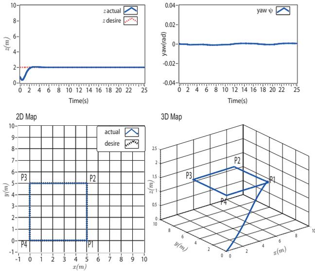
Fig. 4. Simulation result for tracking multi-point. (a) the altitude response. (b) the yaw response. (c) The tracking performance in 2d. (d) The tracking performance in 3d.
