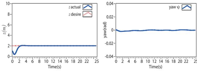
Fig. 10. (a) the altitude response. (b) the yaw response.
