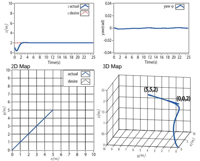
Fig. 7. Simulation result of line tracking. (a) the altitude response. (b) the yaw response. (c) The tracking performance in 2d. (d) The tracking performance in 3d.
