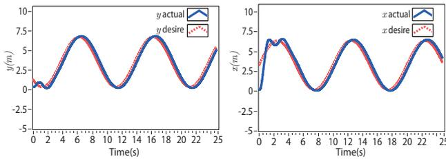
Fig. 12. The position signals generated to track the ellipse trajectory. (a) The desired and the actual values of y. (b) The desired and the actual values of x.
