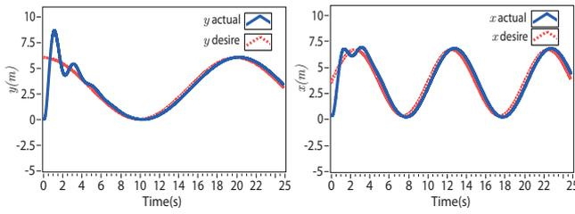
Fig. 16. The position signals generated to track the figure eight trajectory. (a) The desired and the actual values of y. (b) The desired and the actual values of x.
