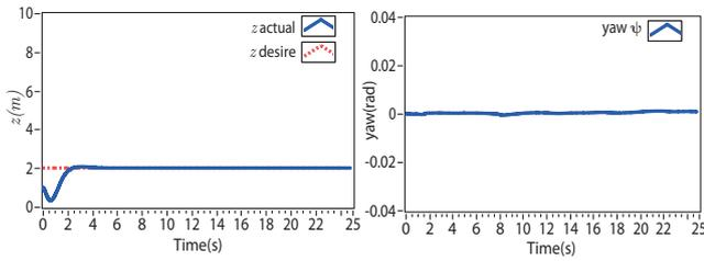
Fig. 18. (a) the altitude response. (b) the yaw response.
