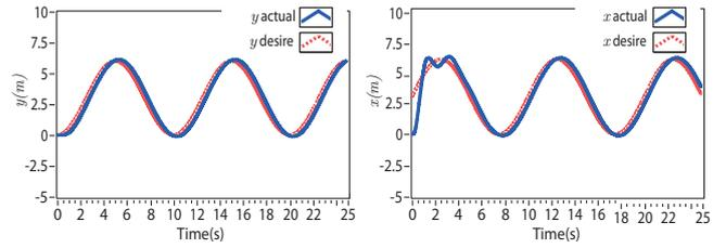
Fig. 8. The position signals generated to track the circle trajectory. (a) The desired and the actual values of y. (b) The desired and the actual values of x.
