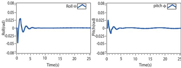
Fig. 17. The attitude signals generated to track the figure eight trajectory. (a) the roll response. (b) the pitch response.
