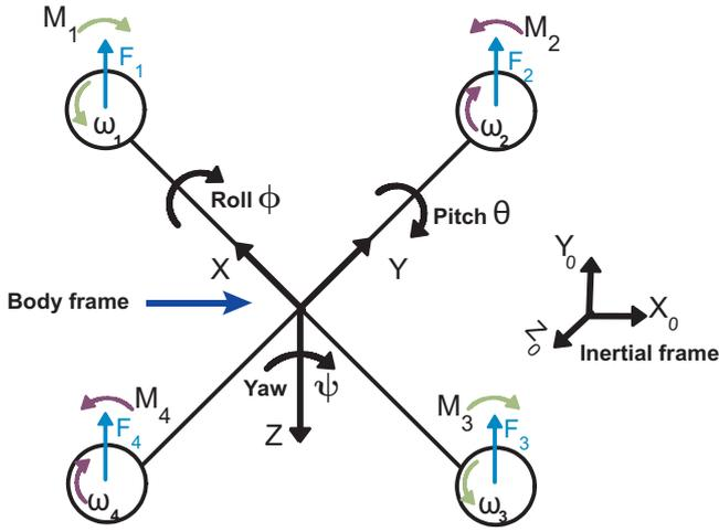
Fig. 1. A typical structure of quadrotor
