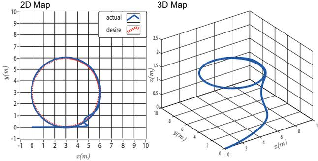
Fig. 11. Simulation result of circular path tracking. (a) The tracking performance in 2d. (b) The tracking performance in 3d.
