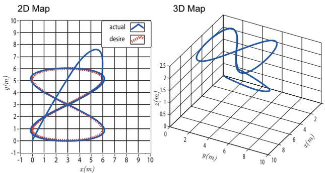
Fig. 19. Simulation result of figure eight path tracking. (a) The tracking performance in 2d. (b) The tracking performance in 3d.
