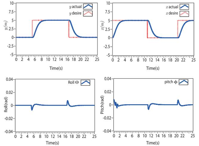
Fig. 3. (a) The desired and the actual values of y. (b) The desired and the actual values of x. (c) the roll response. (d) the pitch response.
