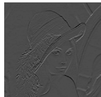
Fig. 4: Edges along Y-axis
