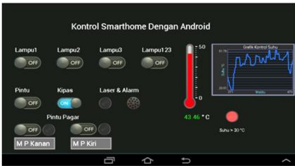
Fig 16. Display for temperature sensor in the room > 30°C
