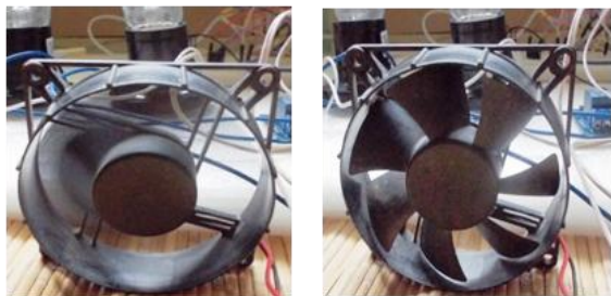
Fig 17. Fan is Active when Room Temperature > 30°C
