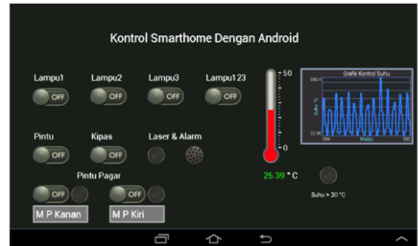
Fig10. Smart Home Control System Using Android Application
