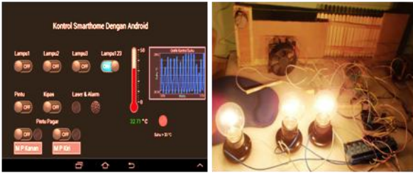
Fig 14. Condition when Lamp123 is Turn On
