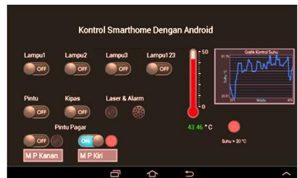
Fig 21. Control to Rotate Left Fence Gate
