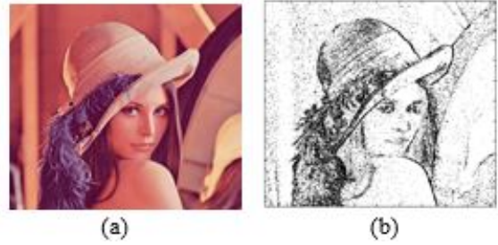
Fig. 3: (a) Lena image. (b)Texture Masking JND_T(I_o) with sliding window 3x3 (with inverted colors)
