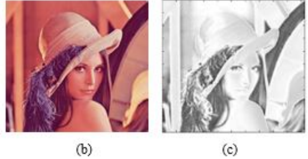
Fig. 1: (a) Visibility threshold relative to the background luminance modeled by Chou [10]. (b) Original Lena image. (c) Luminance masking JND_L(x, y) (with inverted color) obtained for the Lena image. Black parts in the masking correspond to high watermark embedding strength.
