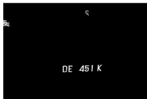
Fig4. Pre-Processed Image after Plate Localization
