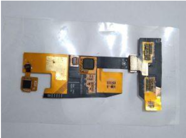
Fig 9: Flexible display with PCB motherboard
