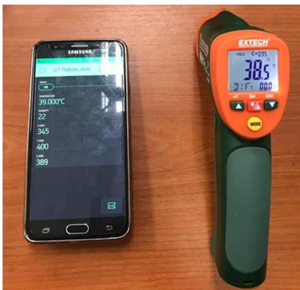
Figure 8: Temperature readings (IoT platform Vs IR thermometer)
