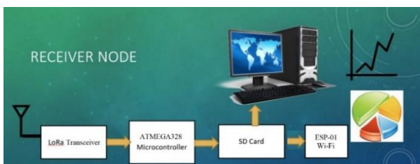
Figure 3: Block Diagram of Receiver Node
