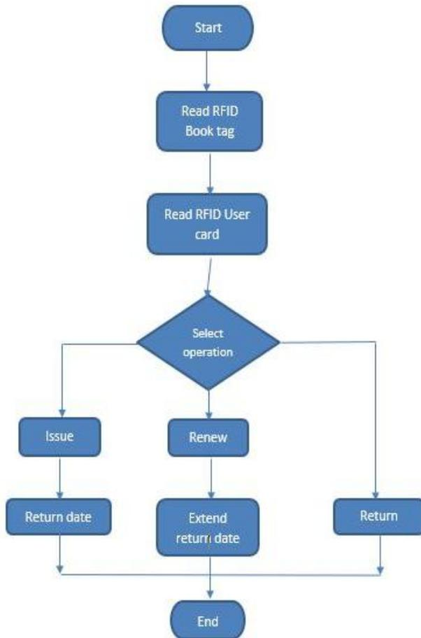
Fig 3: Dataflow diagram
