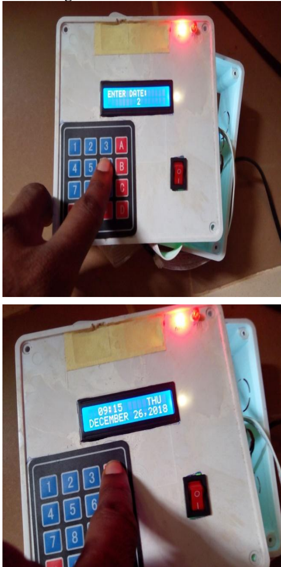
Figure 5: (Top & Bottom) Updating time using Keypad
