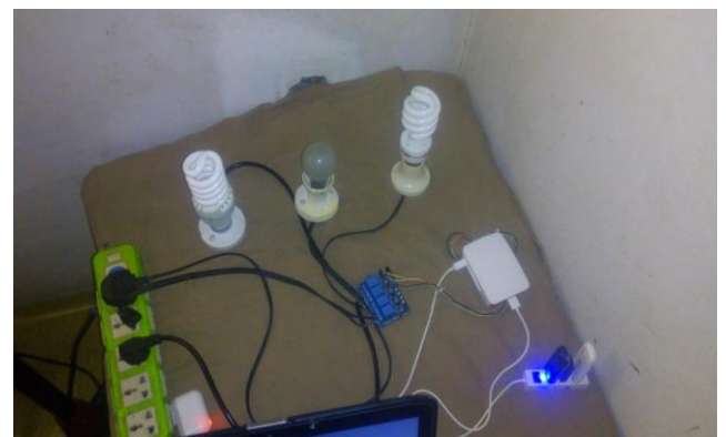
Fig. 2 Connected home appliances with raspberry pi
