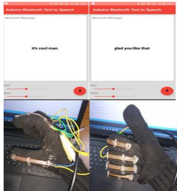
Fig. 7a: Gesture test for “perfect” b. Gesture test for “Likes”
