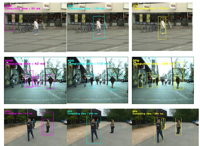
Fig 1. Comparison between HAAR (left), HOG (middle) and DPM (right) applied under three different datasets: TUD-Brussels (top row), ETH (middle row) with 640x480 image resolution, and ESIGELEC (bottom row) with 960x540 image resolution.
