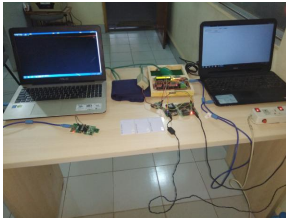
Figure 6: Hardware setup of both transmitter and receiver
