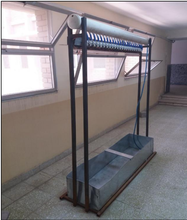
Fig.5. the iron structure with its valves.
