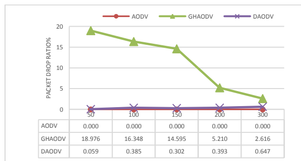
Fig 13: Packet Drop Ratio .vs Number of nodes
