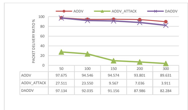
Fig 6: Packet delivery ratio vs Number of nodes
