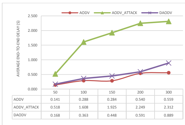
Fig 11: Average end-to-end delay .vs Number of nodes
