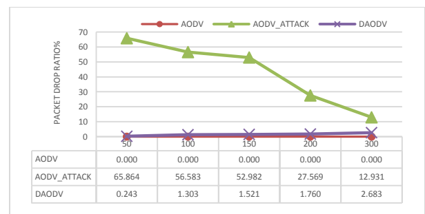
Fig 7: Packet Drop Ratio .vs Number of nodes
