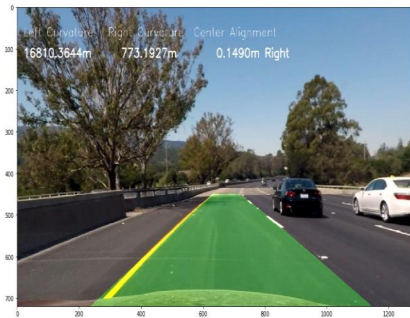
Fig 3.14: Final Output of Detected Lane
