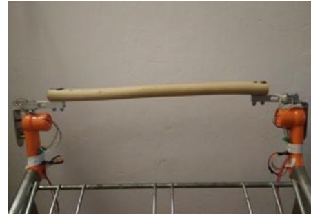
Fig 3: The trolley handle with Load cell mounted
